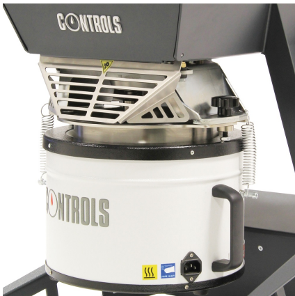
Laboratory asphalt mixer (76-B0702) complete with isomantle heater (76-B0702/HM)
